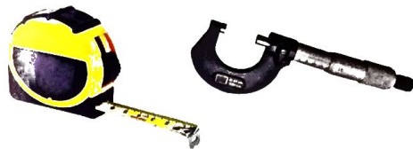
Figure 11 The size of the object being measured determines which unit you will use. A tape measure measures in meters. The micrometer measures in small lengths.
